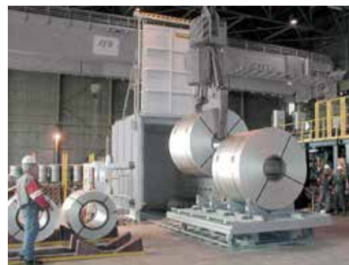
Forced convection bogie hearth furnace for heat-treating coils
