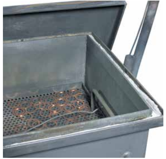
Heat treatment under protective gas atmosphere in a gas-supply box incl. charge thermocouple
