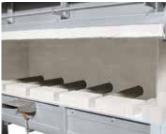
Indirect gas firing with radiation tubes
