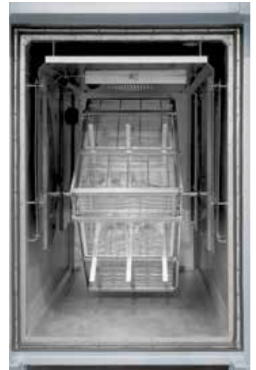
Silicone tempering furnace with tightly welded inner box and rotating rack for the charge.
