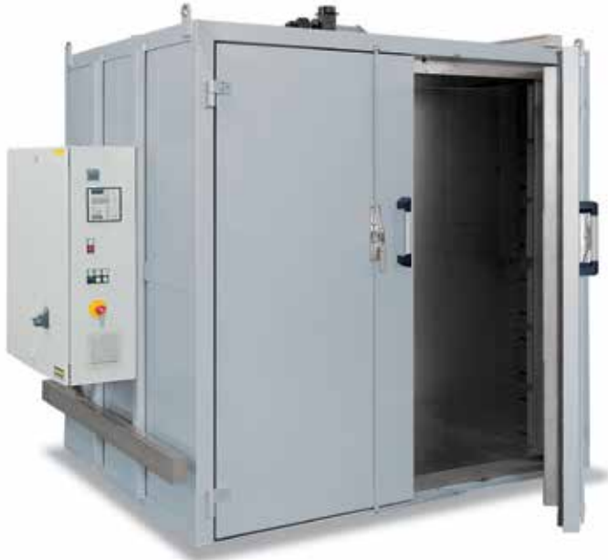
Forced convection chamber furnace N 3920/26HAS
