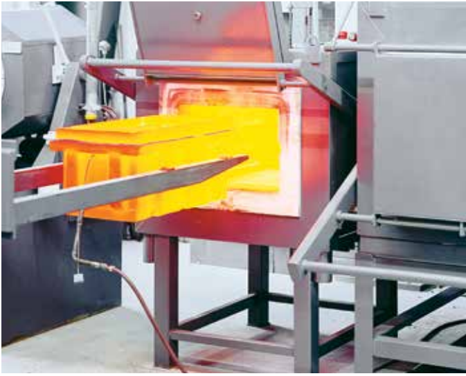
Powder nitriding in an annealing box
