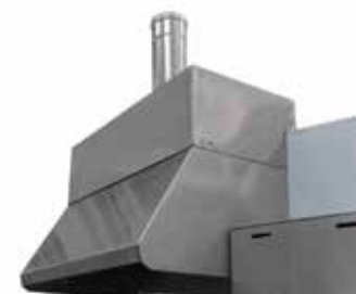
Exhaust hood above charging opening
