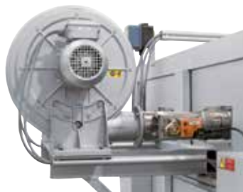
Cooling fan for accelerated cooling
