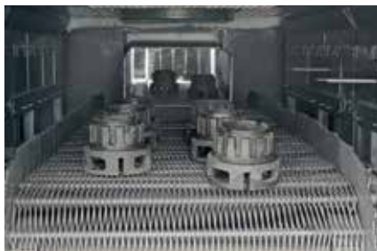
Mesh belt drive in a continuous furnace
