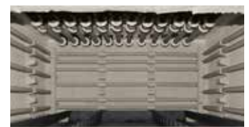
Furnace chamber with optional heating elements in the ceiling when used for preheating of sheetmetal plates
