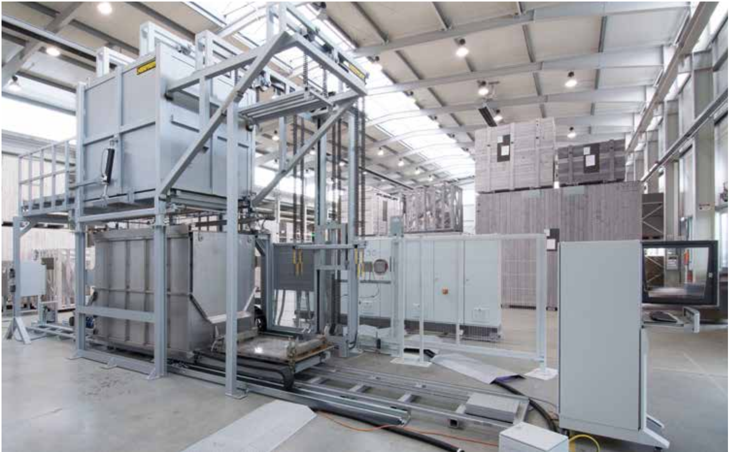
Fully automatic drop-bottom furnace with movable water bath, including holding position for charging and unloading crane
