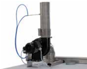
Exhaust port and powerful exhaust fan mounted on the furnace
