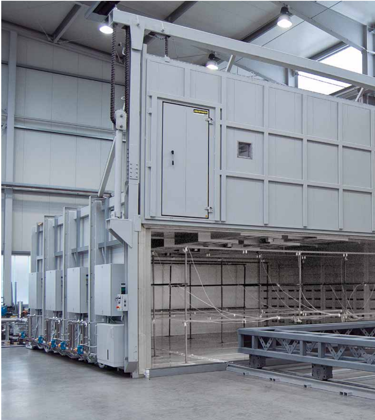
Forced convection chamber furnace N 140000/26AS for curing of composites in vacuum bags incl. pump and necessary connections in the furnace chamber
