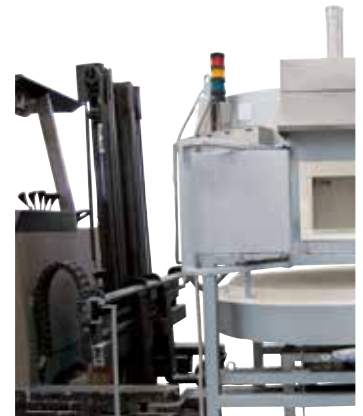
Furnace bottom can be lowered for maintenance purposes
