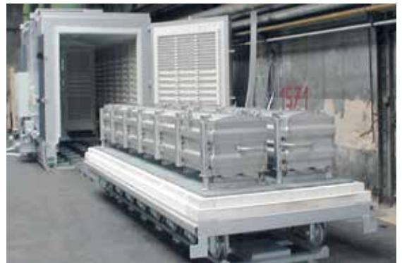
Bogie hearth furnace with gas supply system
