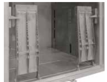
Drive-in ramps at furnaces with bottom insulation for processes which require a good temperature uniformity
