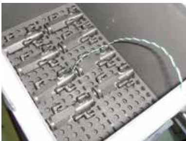
Sintering of MIM titan parts in a VHT furnace
