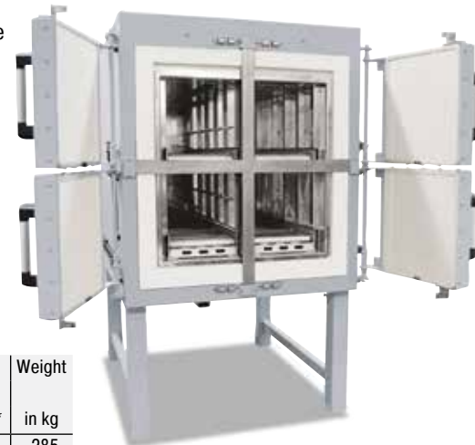
Forced convection chamber furnace NA 500/S with four compartments, each with roller conveyor and individual door
