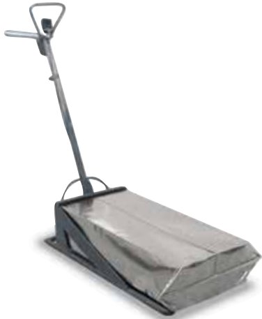
Annealing tray with alloy bag and protective gas inlet
