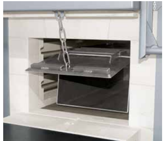
Annealing box with flap which opens together with the furnace door
