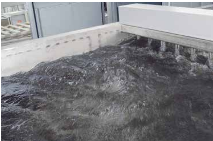
Powerful circulation of quenching medium
