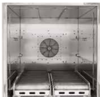
Roller conveyor in forced convection chamber furnace N 250/85HA
