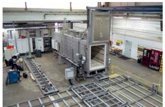
Furnace plant with bogie transfer system in production
