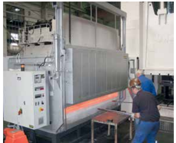
Chamber furnace N 1491/S in production
