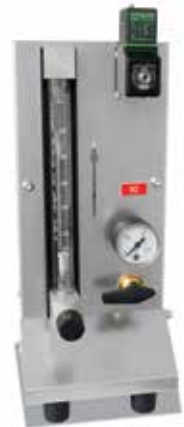
Gas supply system for non-flammable protective or reactive gas with shutoff valve and flow meter with regulator valve, piped and ready to connect
