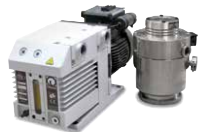
Turbo-molecular pump with booster pump for heat treatment in a vacuum to 10 -5 mbar
