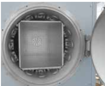
Inside heating in retort furnaces NRA ../06
