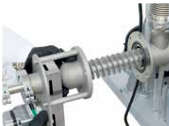
Screw-conveyor with adjustable speed
