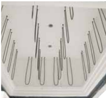
Heat from all sides and between the stack to optimize temperature uniformity
