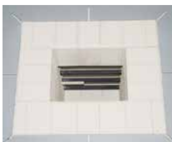
Two-side heating with SiC rods
