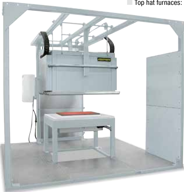
Top hat furnace H 240/S. Table accessible from four sides for welding quartz glass constructions by vertical and horizontal moveable top hat
