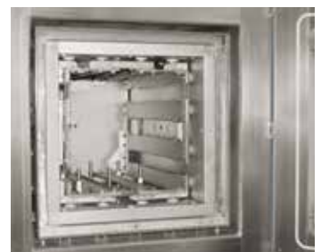
Tungsten heating chamber
