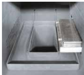
Insulated cover of the salt-bath
