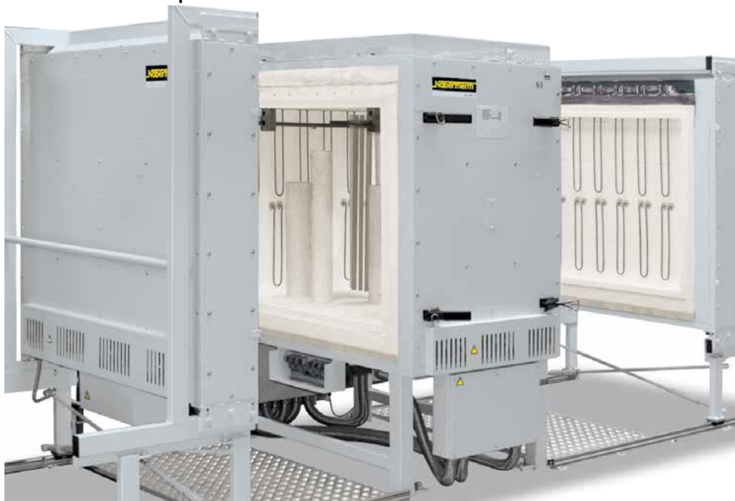
High-temperature furnace HT 1000/17 with two movable door segments and fourside heating for sintering hanging ceramic tubes up to 1700 °C
