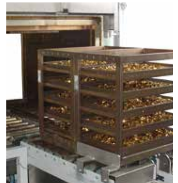
Continuous furnace for bulk materials in baskets
