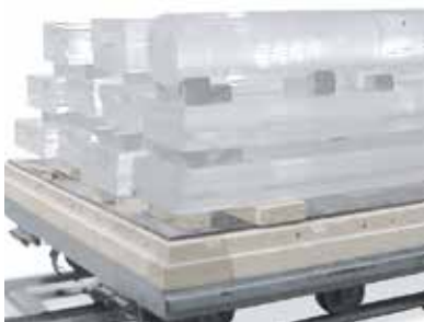
Bogie hearth furnace for tempering quartz rods
