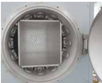
Inside heating in retort furnaces NRA ../06
