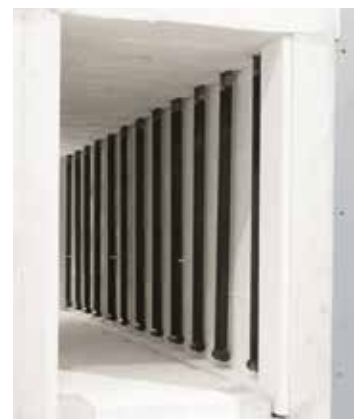
SiC rod elements on both sides of the bogie hearth furnace
