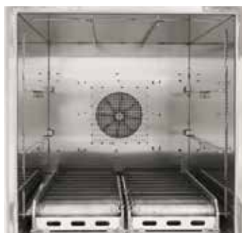
Roller conveyor in forced convection furnace N 250/85HA
