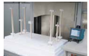
Measurement setup to determine the temperature uniformity in a high-temperature bottom loading furnace
