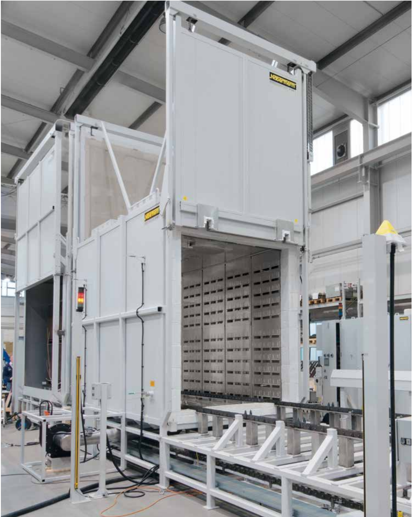
Continuous furnace plant for working temperatures up to 260 °C with integrated cooling station
