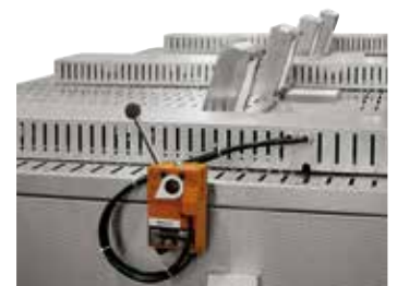
Motor-driven exhaust air flaps as additional equipment
