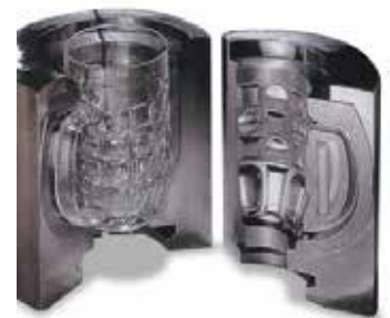
Production moulds for beer glasses
