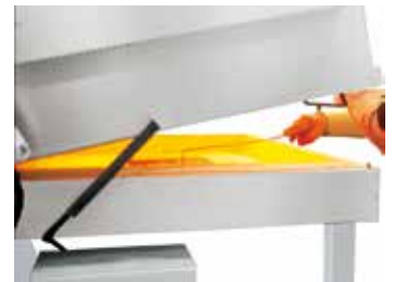
"Combing" in a fusing furnace GF 240
