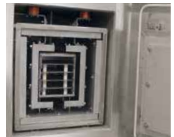
Molybdenum heating chamber
