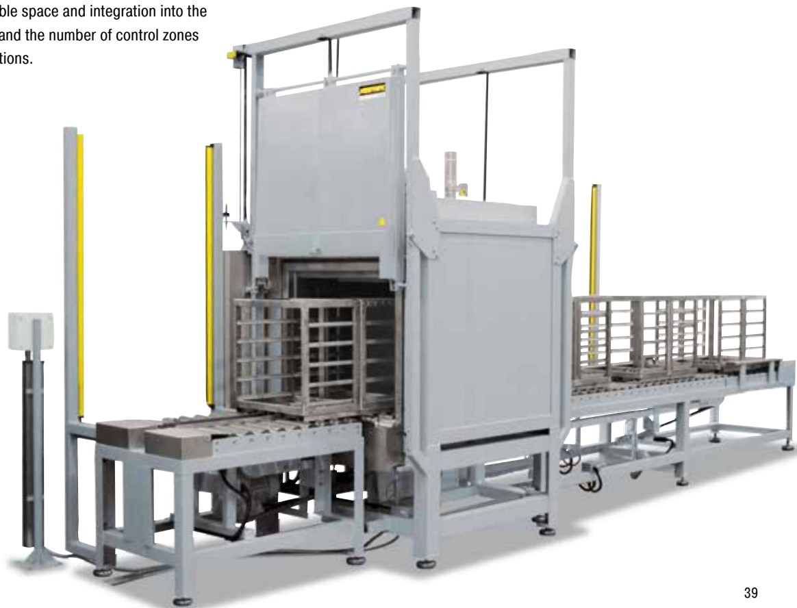
Continuous furnace for bulk materials in baskets
