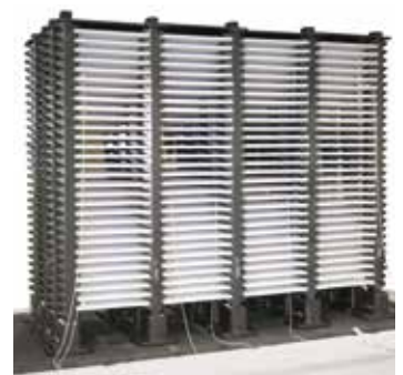
Kiln furniture for small ceramics components
