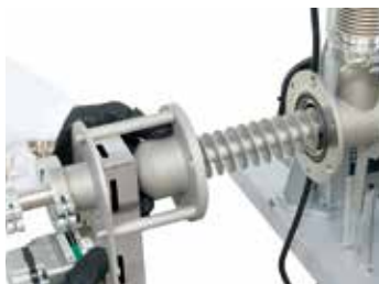
Screw-conveyor with adjustable speed
