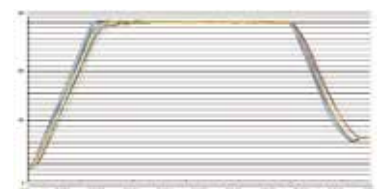
Temperature recording in accordance with EN 14179-1
