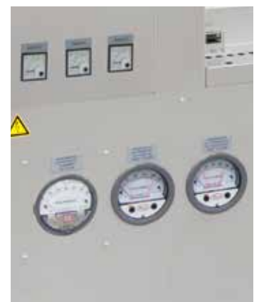
Display of pressure and volume flow with debinding package DB200
