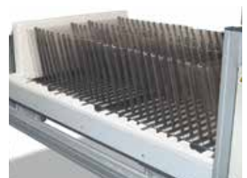
Charging trolley for disc coating
