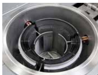
Cylindrical retort with tungsten heating
