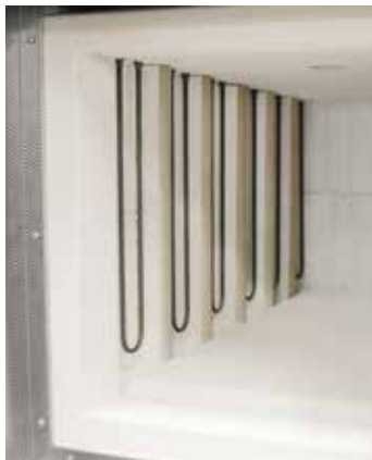
Protection of heating elements against mechanical damage
