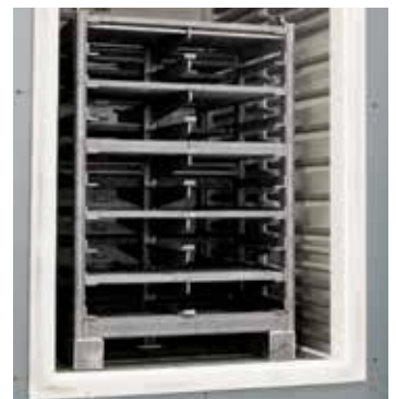
Charging trolley for chamber furnace N 2200
