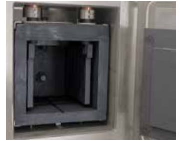
Graphite heating chamber
