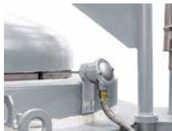
Thermocouple for melting bath control
