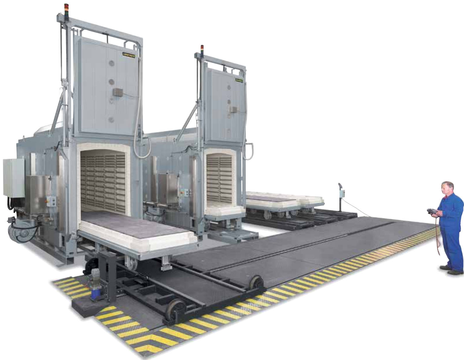
Combi furnace system consisting of two furnaces W 5000/H and two additional bogies incl. bogie transfer system and incl. necessary park rails
