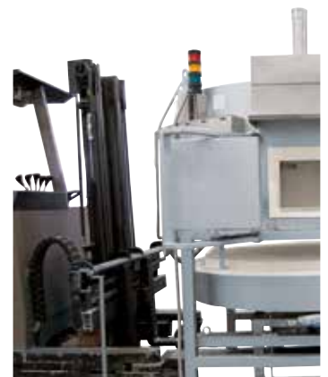
Furnace floor can be lowered for maintenance purposes
