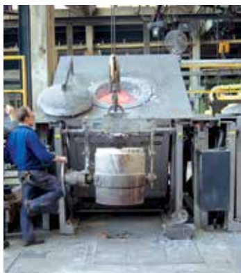
Charging of transport ladle with K 360/12
