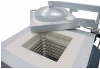
Crucible Pulling Feature with swinging collar plate
