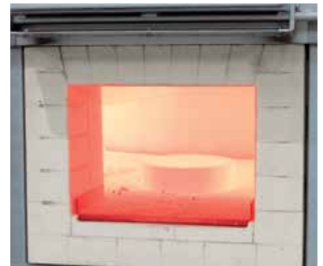
Pre-heating of steel rings for forging
