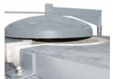
Swing lid with good sealing to collar plate to avoid heat loss over the crucible opening
