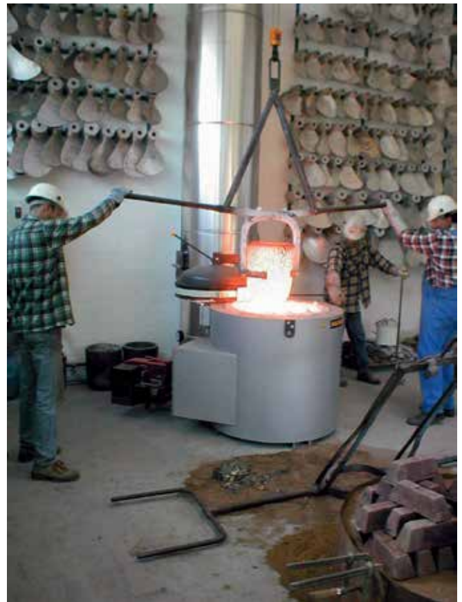
TB 40/14 with crucible pulling device
