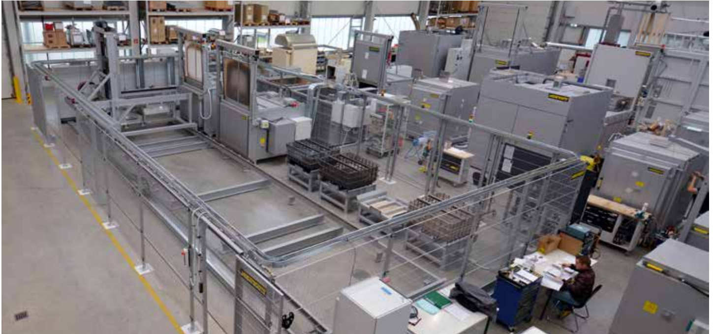
Fully automated tempering system with two chamber furnaces, quench bath, conveyor system, and parking spots for four charge baskets
