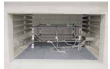
Measurement set-up in an annealing furnace
