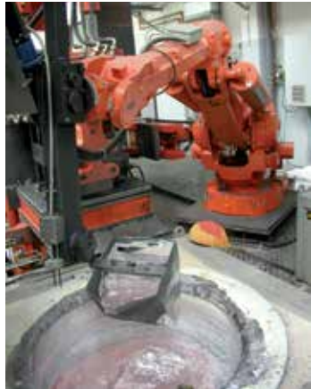
Bale-out of T 650/10 with robot
