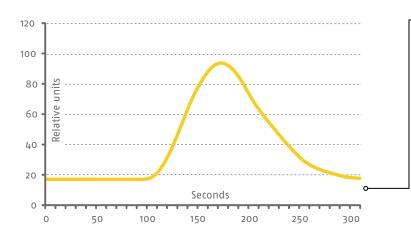
Reliable determination of 100 μg / kg sulfur in a standard thanks to an outstanding low baseline noise and drift.
