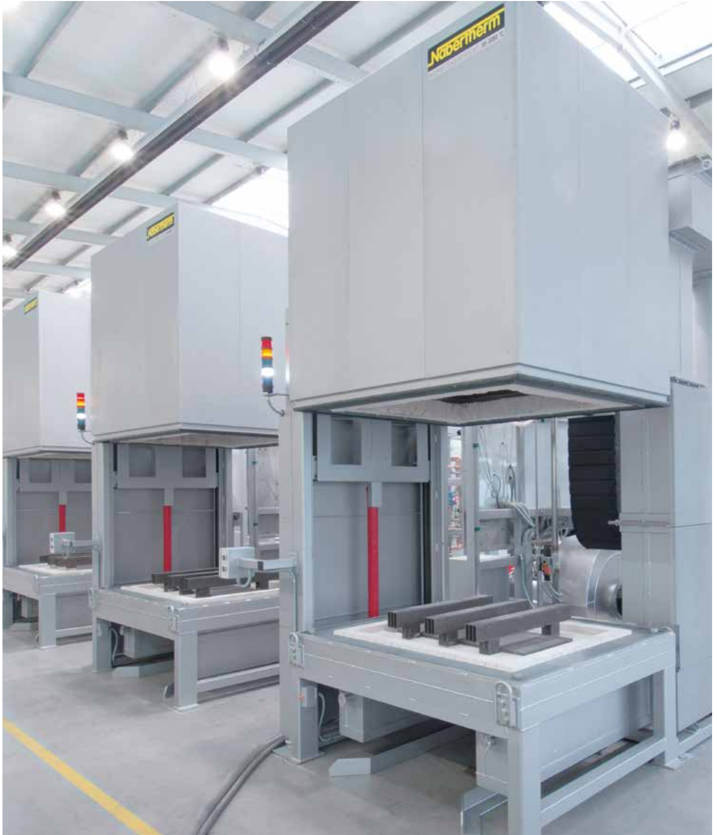
Production plant, consisting of 3 lift-top furnaces HAS 1560/95S with sealed housing for operation with nitrogen. Including air/gas heat exchanger for reduced cooling times
