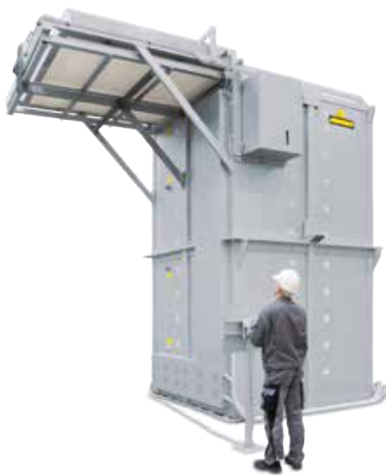
Pit-type furnace S 11988/S with rolling lid
