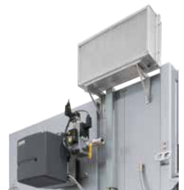
Direct gas-firing at a chamber dryer
