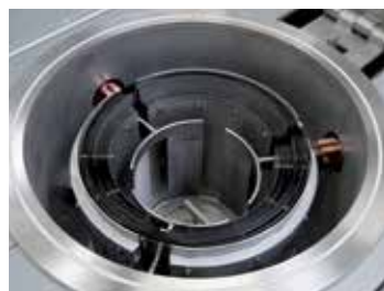
Cylindrical retort with tungsten heating
