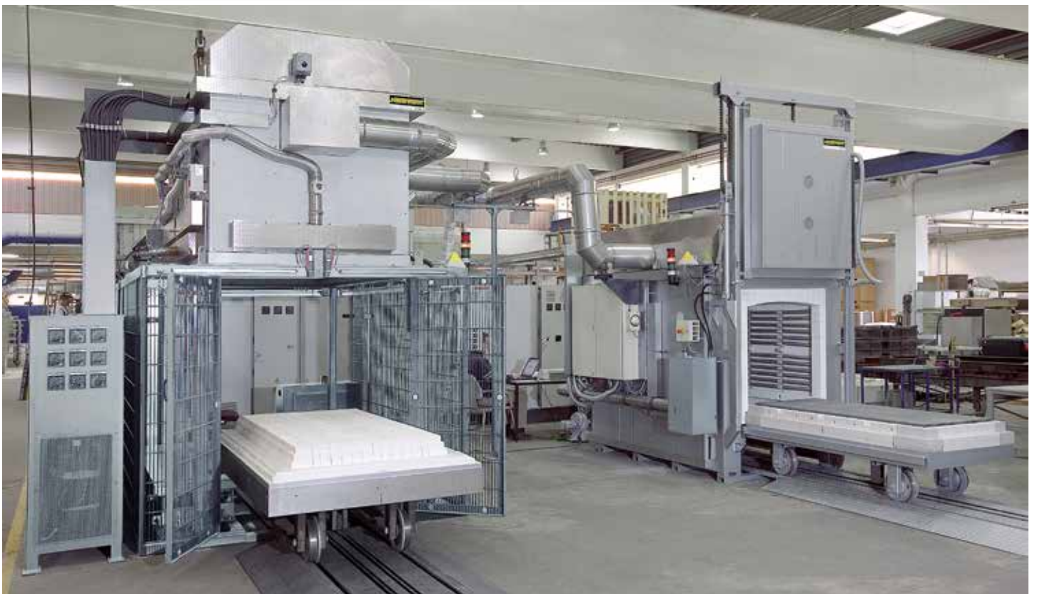
Production system consisting of a bogie hearth furnace for debinding and a high-temperature furnace for residual debinding and sintering with shared catalytic afterburning system
