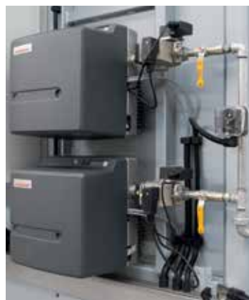
Gas burners for furnace heating and thermal afterburner
