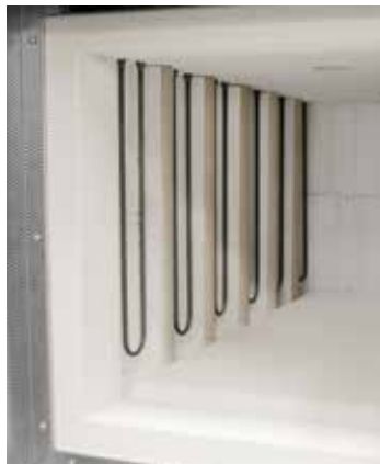
Protection of heating elements against mechanical damage
