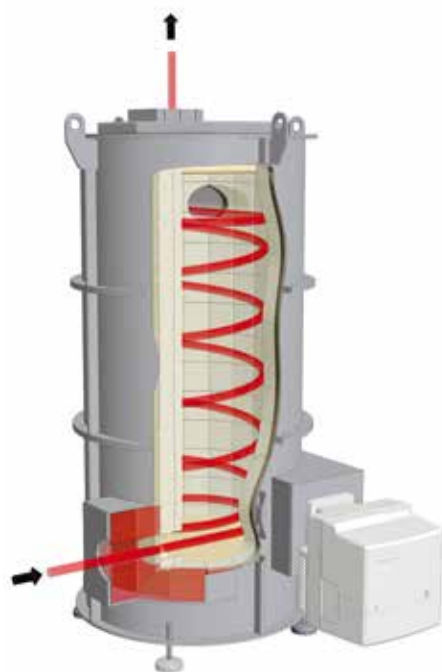
Scheme of a thermal afterburner system
