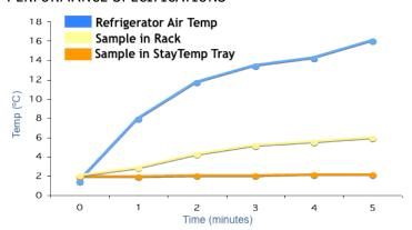
Samples stay at temperature even when refrigerator door is left open for 5 min. With the refrigerator door open for 5 minutes, a 5 ml liquid sample (water) remained at the set temperature (2 °C ±0.5 °C) when stored in a 4 L StayTemp™ equipment Tray. When the same sample was stored in a standard rack, it warmed up to 6°C. The sample temperature was monitored over time. Data represent temperature measurements recorded by a single temperature probe. Values represent ±S.E. (n=3).
