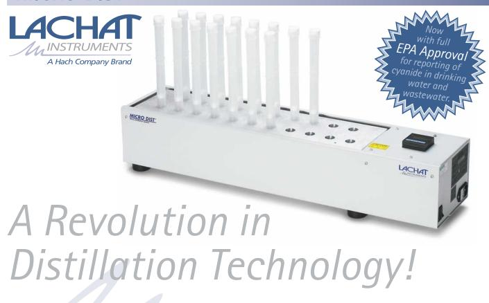
With the MICRO DIST system from Lachat Instruments, you can now distill up to 21 samples for cyanides, sulfide and ammonia in 30 minutes; and phenolics and tritium in 90 minutes. MICRO DIST eliminates the need for bulky, expensive, clumsy and time-consuming glassware-based distillation units while accommodating liquid and solid samples.
