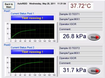
As soon as maximum stable pressure is reached the test stops automatically and saturated vapor pressure (RVP) is recorded.
