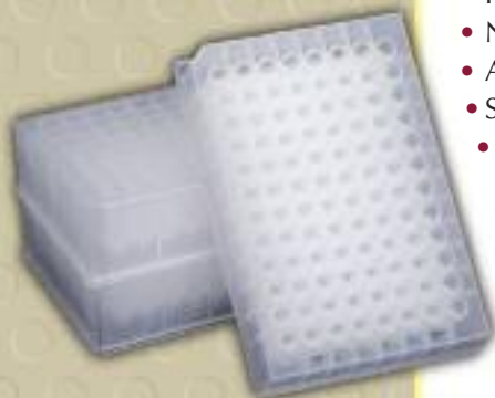
96-Well SpinColumn high throughput sample prep applications, volumes 25 µl to 150 µl. See pages 91 and 92.
